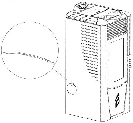
Remove the micro-connections shown in the illustration
