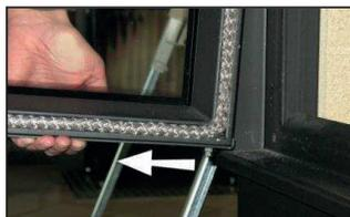
5. Now allow the door to drop down a little so that it comes away from the upper guidance pin and can be removed.
