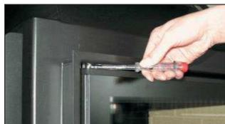
2. Swing the door open. Then tighten the Allen screw on the lower hinge with a 3 mm Allen key.
