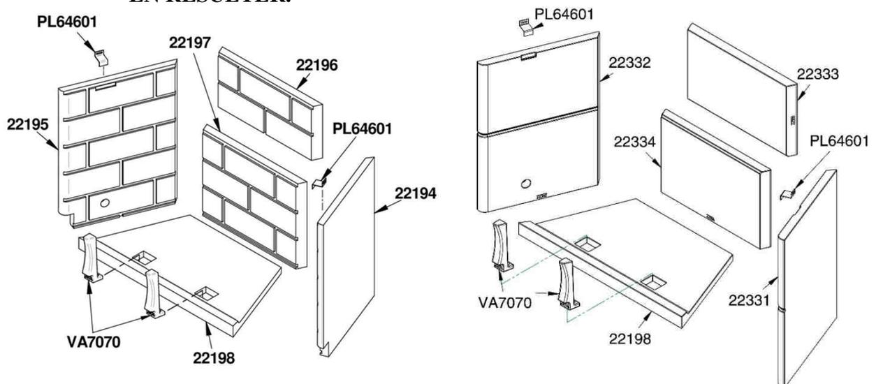
Figure 41: Replacing Antoinette refractory panels
