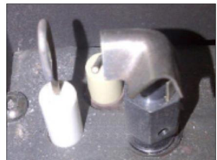
Figure 25: Correct Pilot Position
