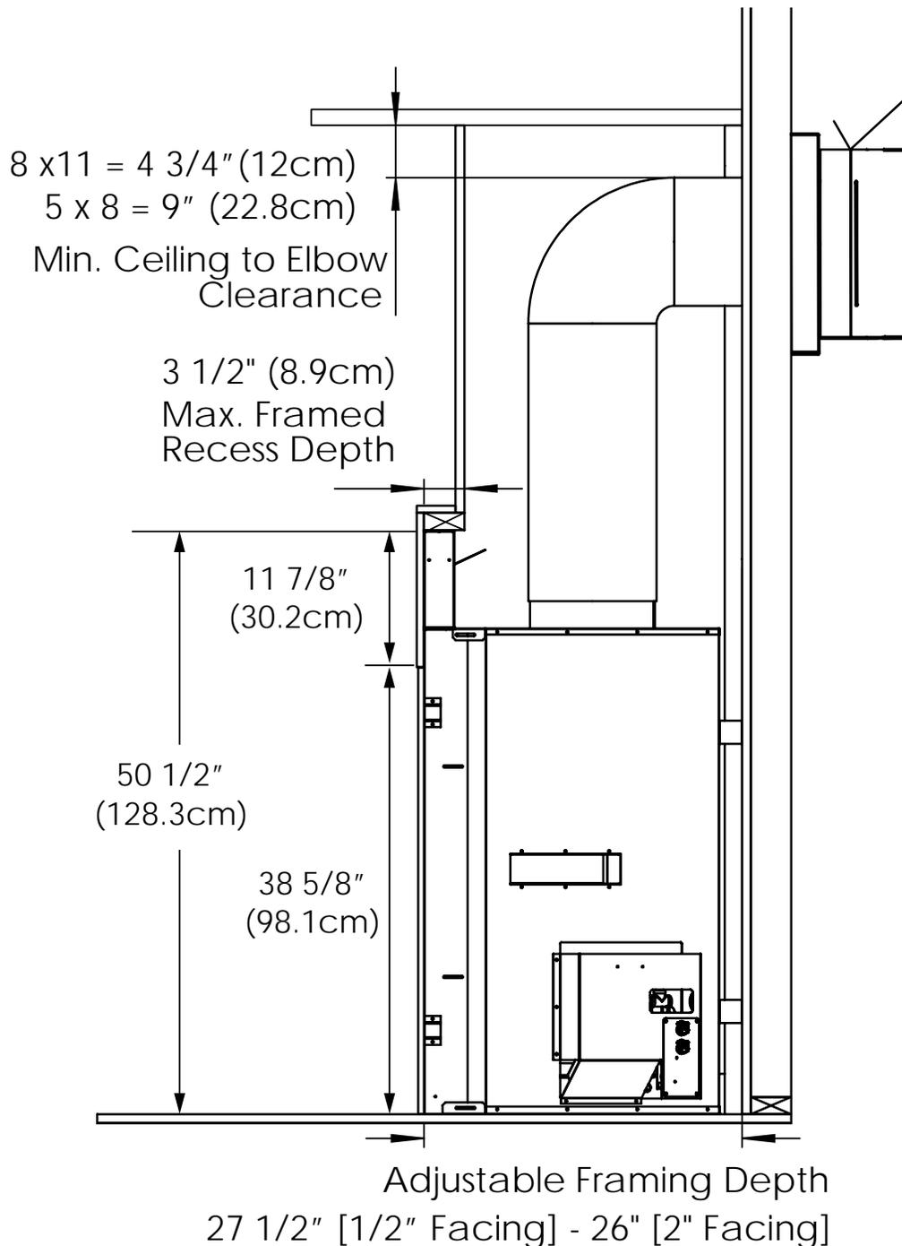
Figure 50: Recess Installation
