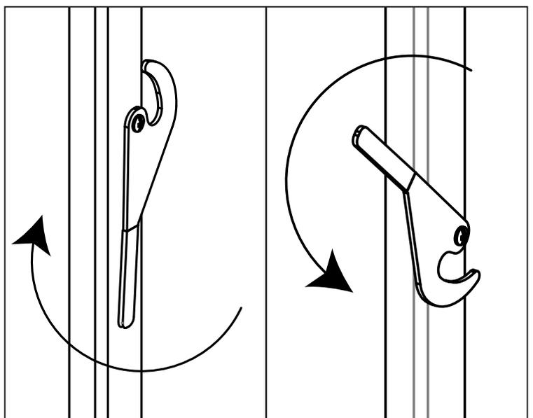
Figure 7: Door Hook Unlock (Left) and Lock (Right)
