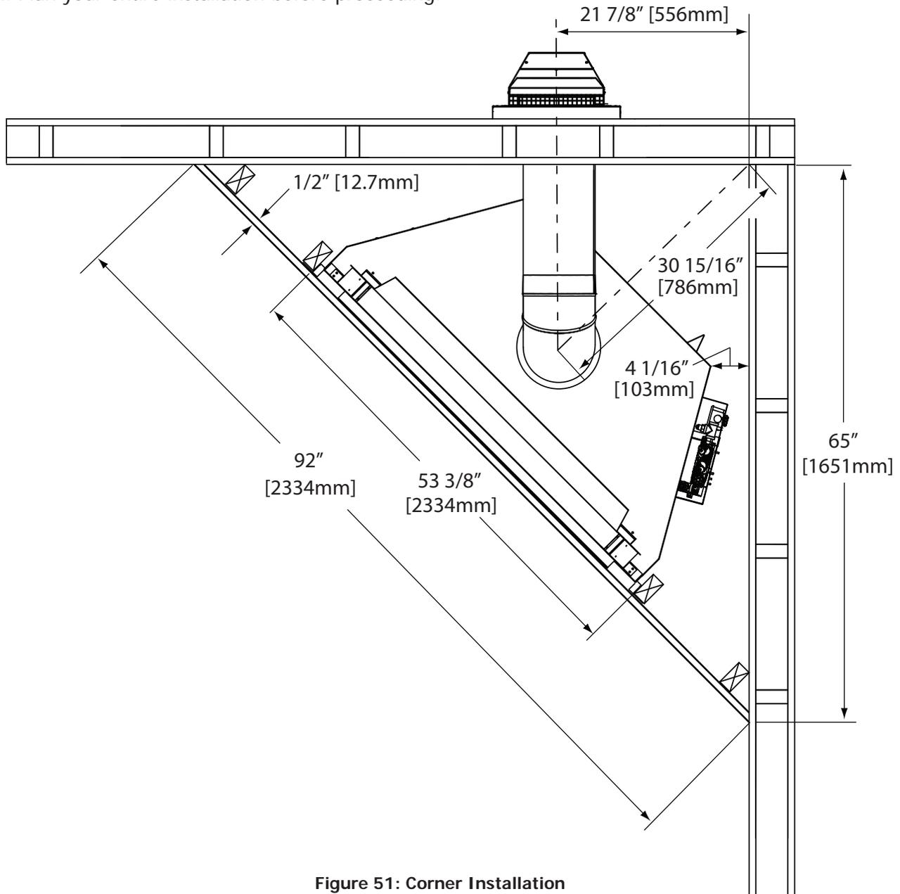
Figure 51: Corner Installation
