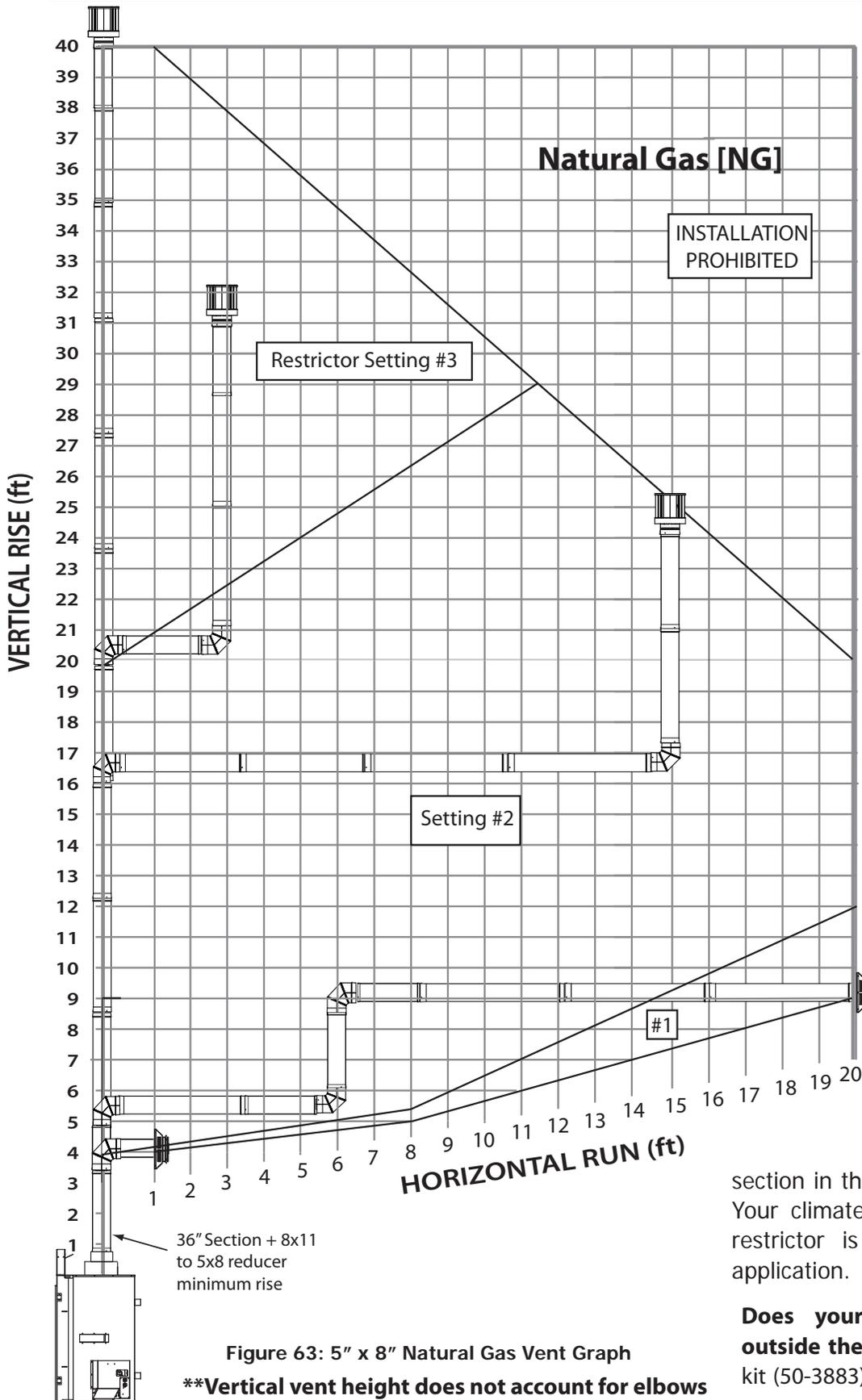
Figure 63: 5" x 8" Natural Gas Vent Graph
