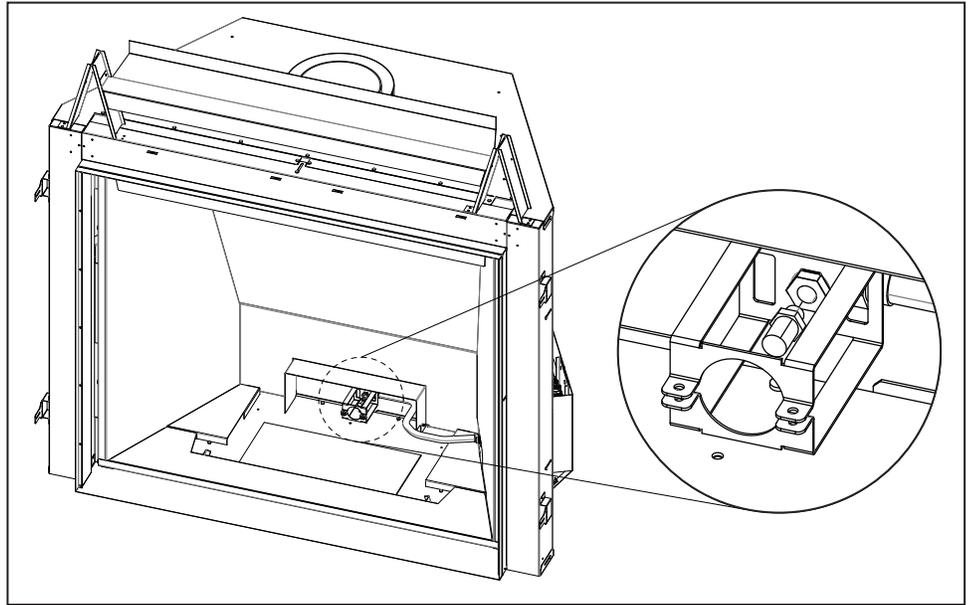
Figure 22: Orifice Location
