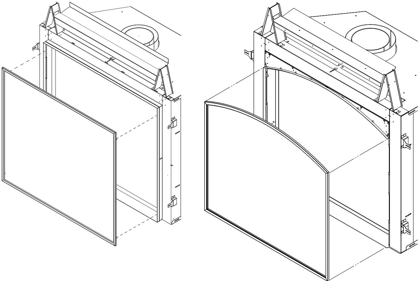
Figure 4: Safety Screen Removal (U44I and U44I-A models)
