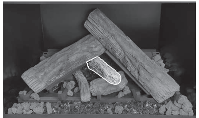
8. Place log 5 underneath log 1 and on of log 3, be careful not to place it too close to the right burner or it may cause sooting.
