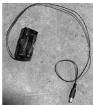
Figure 11.2 - Bloc-piles de secours
