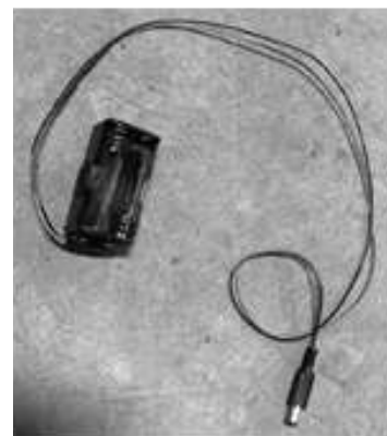
Figure 11.2 - Bloc-piles de secours
