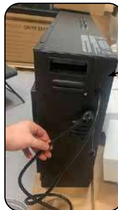
Wire Harness & Cover Plate Reinstalled.
